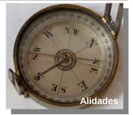
communicate with two readings on their alidades and where they intersected, thus giving a precise fire location. The lookouts would dispatch the fire location along with the color of the smoke, the approximate size of the fire and the distance from the towers. This enabled fire response crews with information for fire location and time needed to travel to the fire. What an important and valuable tool the Central Fire Tower provided.
